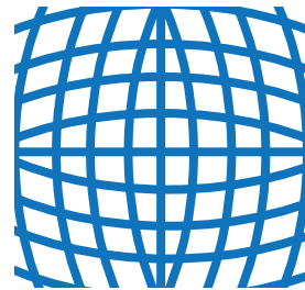
Positive radial distortion "barrel"
