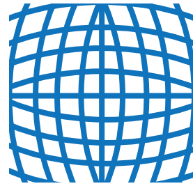
Positive radial distortion "barrel"
